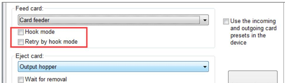
A. When the "hook mode" and "retry by hook mode" are not chosen, the card feeding by roller only.
