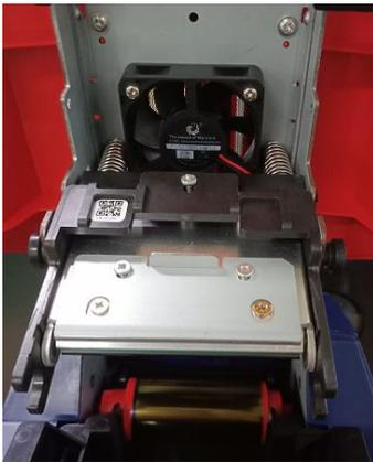
Step 6: Enter the new print head serial number into the driver. Failure to enter may result in an abnormal print.
