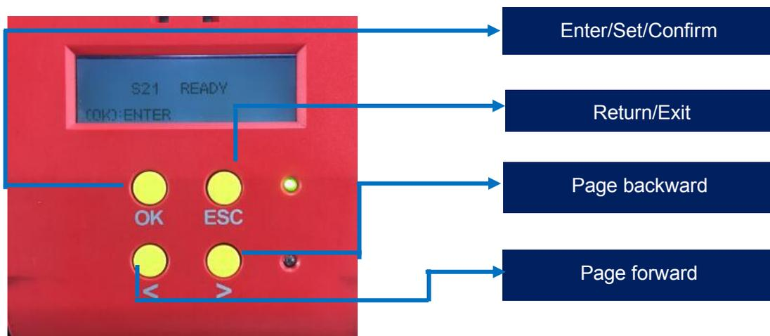
Step 3: LCM show "Clean function" press "OK" one time. Then LCM will show "Open the cover".
