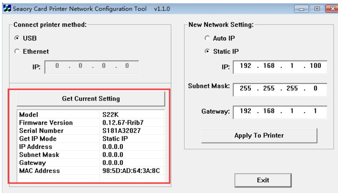
Step 4: Click “Static IP”, type in internet IP address, subnet mask, gateway information. Then click “Apply to card printer”, you will see success dialog box. That means the network setup successfully.
