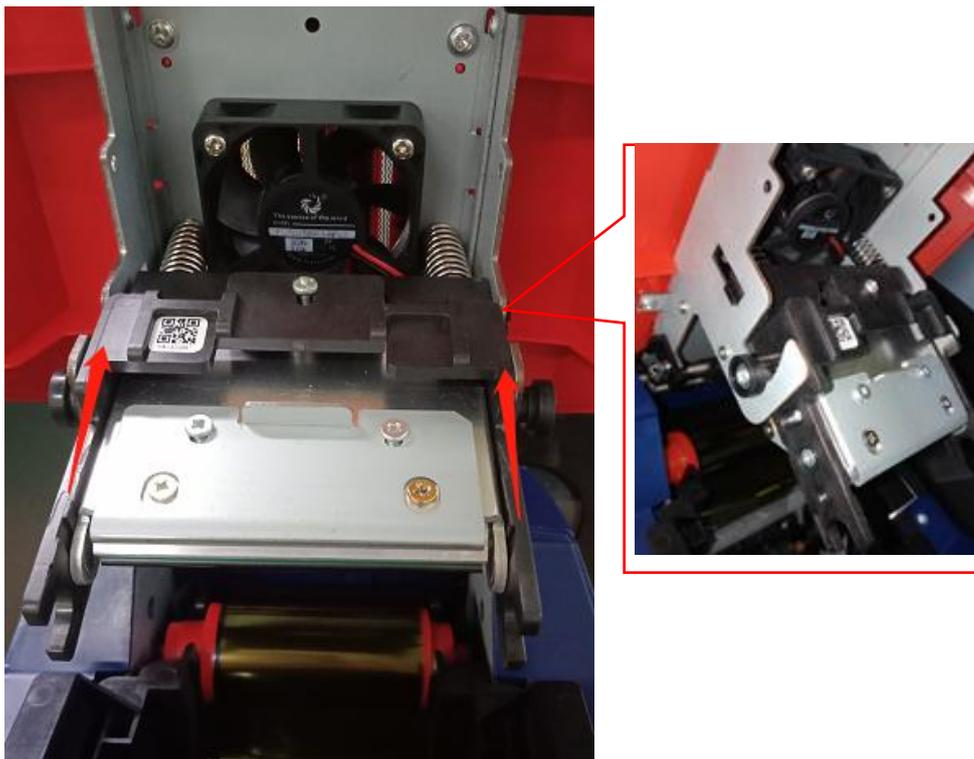
Find the wiring and pull it out from the wiring plug with your hand.
