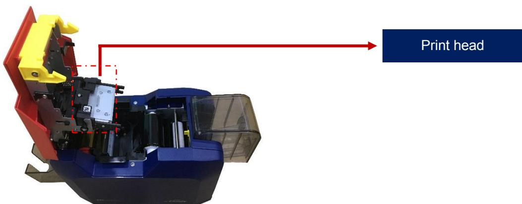
Step 3: Wipe the print head one direction, from left to right or right to left with cleaning stick. Do not wipe back and forth. Generally wipe 3-5 rounds will be ok.
