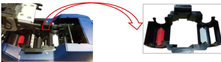
Step3: Remove 3M hyaline layer on cleaning roller surface, take the cleaning roller's both sides by hand. After pushing into the mounting position, gently press down.
