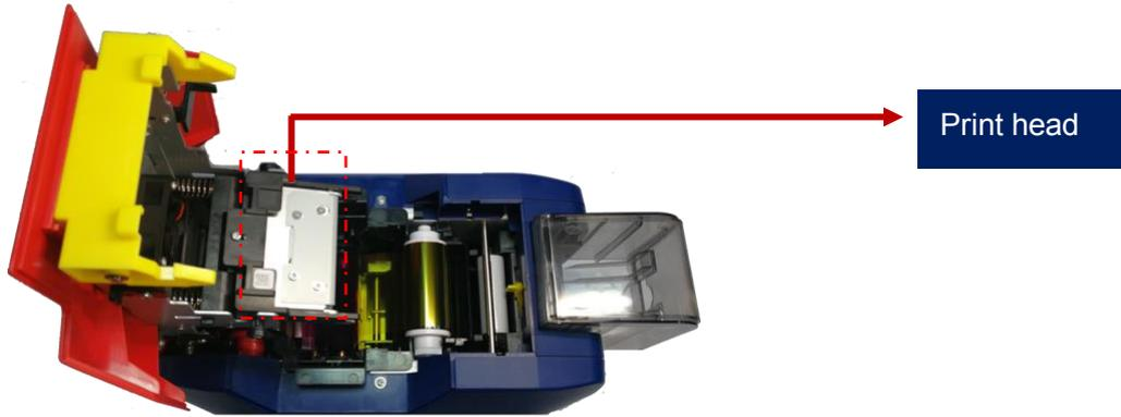
Step 3: Look closely at the mounting structure on both sides of the print head.
