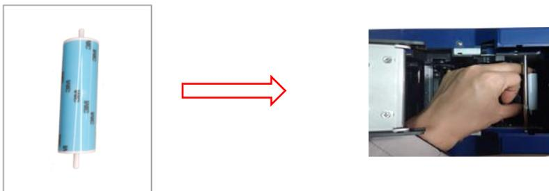
**i** The purpose of cleaning roller is to absorb the dust on the card and card feeding path, improve the printing effect.
