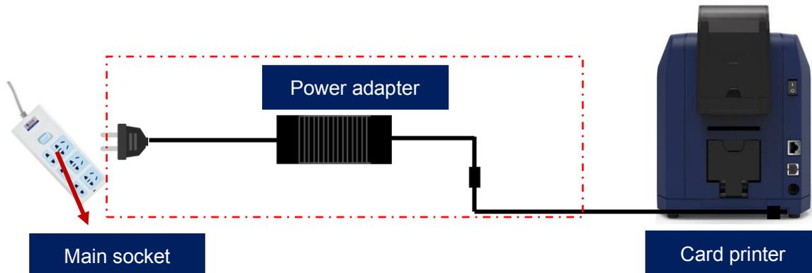
**i** To ensure the card printer work stably, please use Seatory original power adapter.
