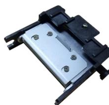
Step 2: Turn off the card printer, open the upper cover and find the print head show in below picture.
