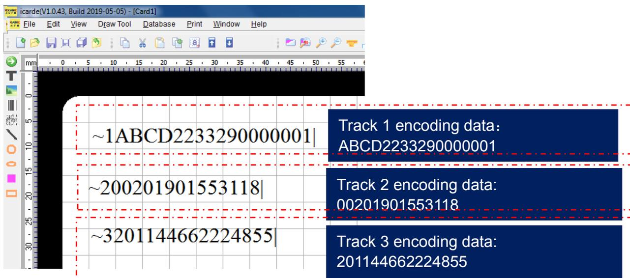
"~1" means track 1 , "~2" means track 2, "~3" means track 3. "|" means stop code.
