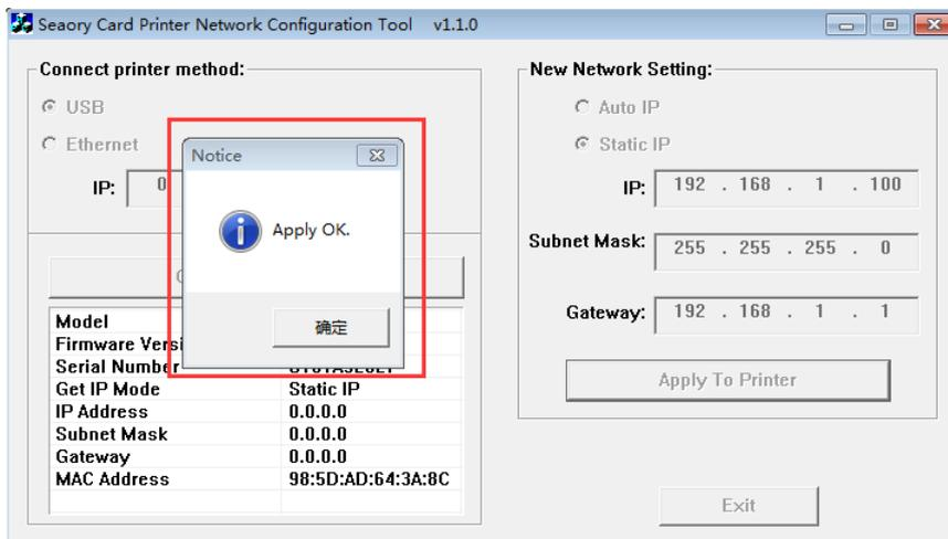
**i** After setting successfully, you can use the Ping network command to test the result.
