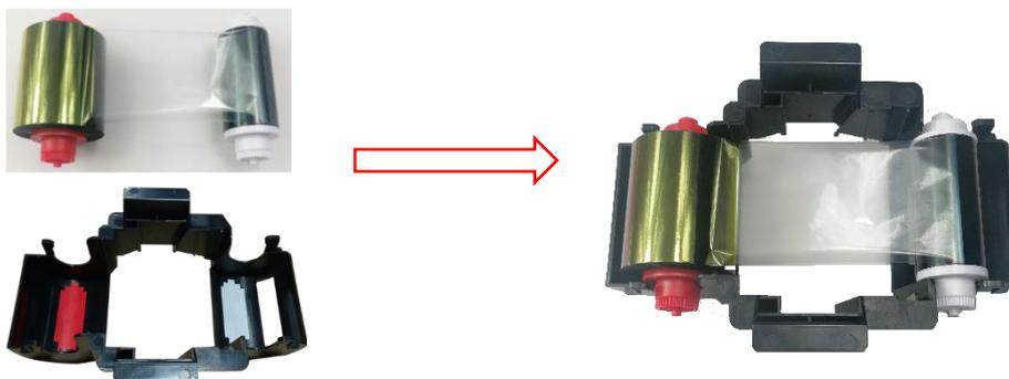
**i** Red roller supply with unused ribbon. White roller supply with used ribbon.
