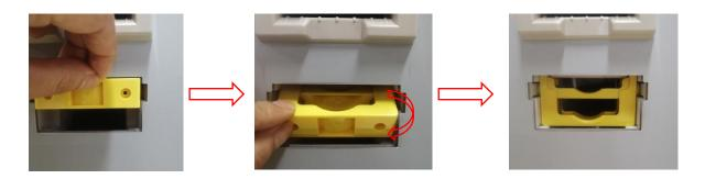
After above steps are completed, then close the upper door to complete the installation of the cleaning module (bottom).
