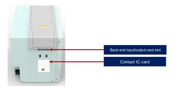
• The ISO7811 standard card should be inserted strictly according to the card direction in the picture above, so that the magnetic stripe position is at the bottom left of the card, which is consistent with the ATM card insertion rules. If you only need to print and do not need to encode magnetic stripe data, there is no requirement for the card direction, it can be customized according to your needs.
