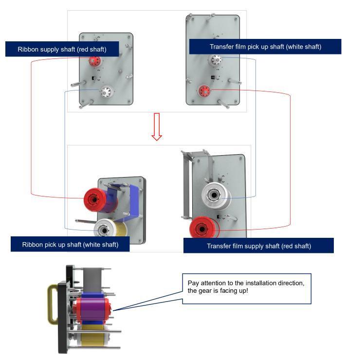
Supply shaft: the red end is the supply shaft, unused consumables (ribbon or transfer printing film);
