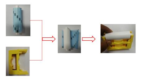
After tearing off the 3M adhesive layer on the surface of the cleaning roller, hold the two ends of the cleaning roller with hands, push them to the installation position and gently press down to lock until the ends do not fall off.
