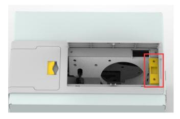
The function of the cleaning roller is to absorb the dust and foreign matter entering the card roller, indirectly stick to the dust on the card surface to improve the printing effect.
