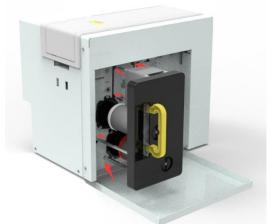
(2) Align the post of the ribbon holder with the hole as shown in the picture above and gently push it into the card printer.
