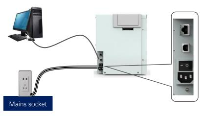
Ethernet communication interface installation: RJ45 network interface ,568B connection mode.
