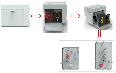
Warning: When card printer shipped from the factory, there will be placed a piece of sponge paper next to the print head, please take it off before use or the power on test, otherwise it may cause damage to the printhead. Operation steps are as follows. As shown in the picture below, follow the operating guidelines to remove the right ribbon holder, and then remove the sponge paper as shown.
