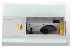
Note: The purpose of the cleaning roller is to absorb the dust on the card and improve the printing performance.
